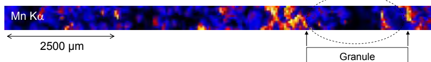
Figure 1. Mn XRF maps for fluid Mn and granular Mn treated in experimental cells. Fertilizer granule extracted from soils clearly shows the presence of concrete-like precipitate adjacent to the granule.
