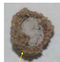
Concrete like outer shell, soil + precipitates
