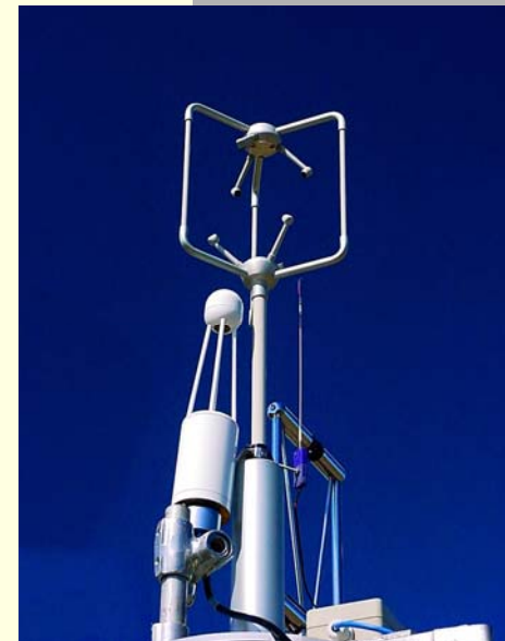
Close Up of Eddy Covariance Flux Sensors
