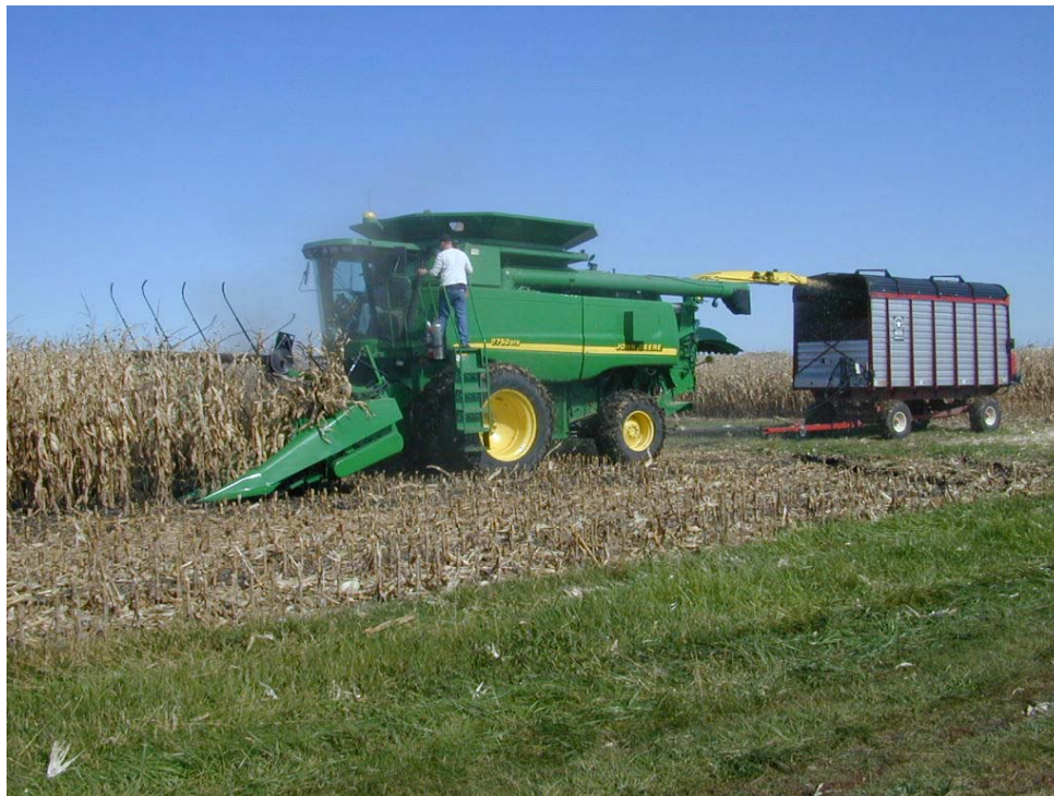
Figure 1. Single-pass corn grain and stover harvest operation near Ames, IA.
