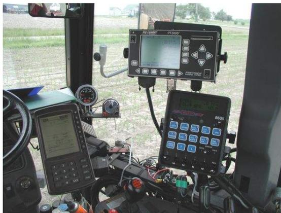
output the target rate to the Hiniker rate controller via a serial cable. The rate controller recognizes the rate change and makes adjustments to valves to increase or decrease the applied rate. Finally, the actual applied rate is read by the controller and sent back to the computer on the serial cable where it is logged by the AgLeader system to a removable data card. This process repeats every 1-2 seconds.
