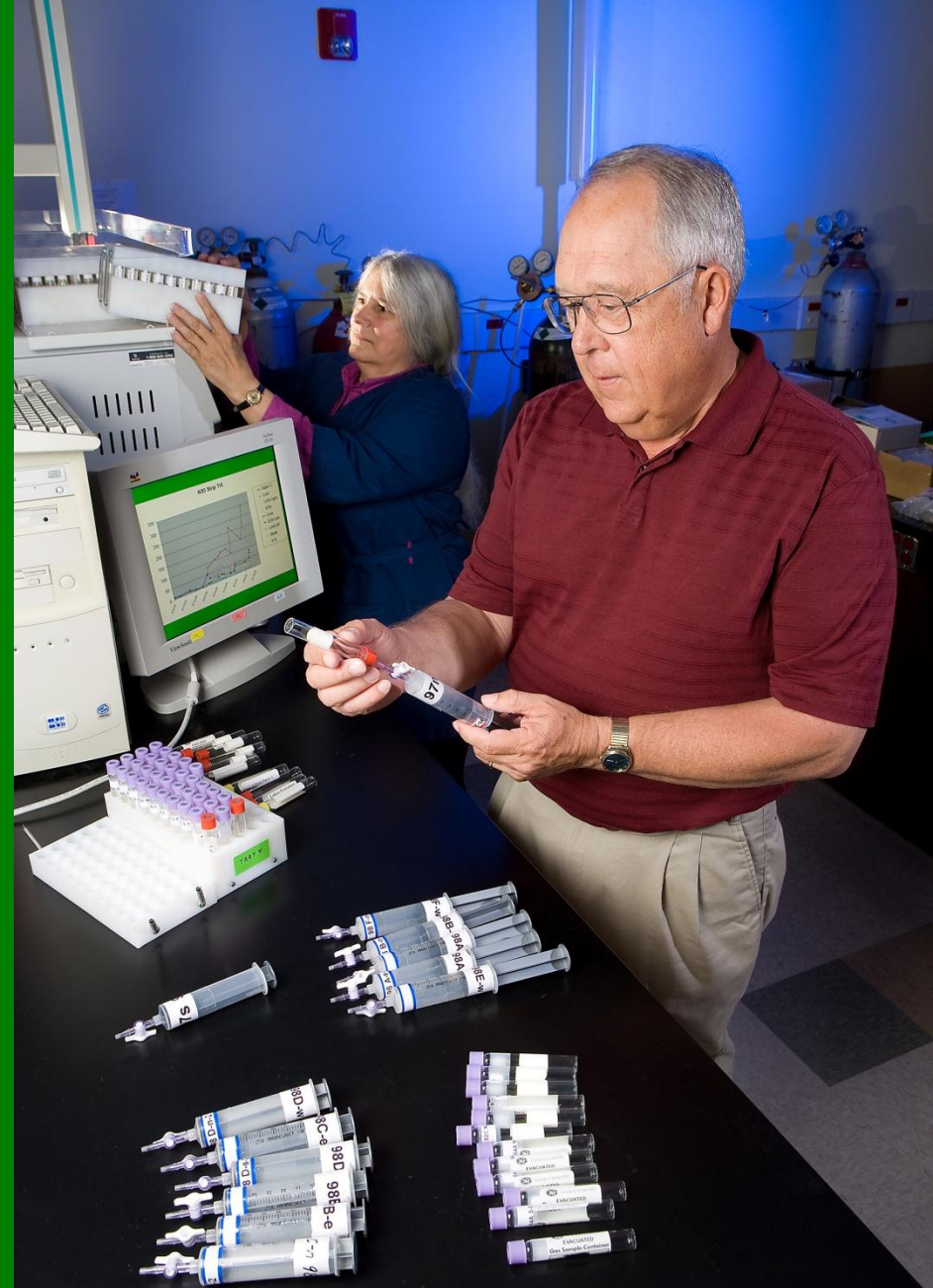
Injecting field gas samples into vials for analysis on Varian 3800 GC.
