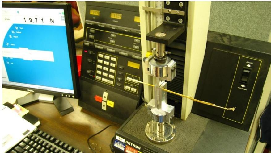
Figure 2. Shear box attached with load cell that hooked with a computer.
